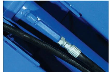
The inverted deck cylinder is continually self-bleeding, reducing internal corrosion and increasing velocity fuse efficiency.
