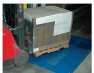
For high-volume operations with more demanding usage levels, Blue Giant offers assured motion float, a 4" (101 mm) maintained deck tilt, as an optional alternative to the standard fixed rear hinge.
