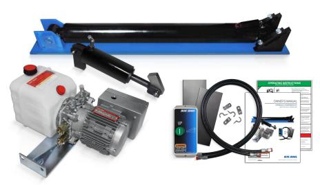
Deck and lip operation is accomplished quickly and easily using a push-button control station: no more chain-pulling or "walking" down the deck. A hydraulic velocity fuse replaces the mechanical safety legs, adding an extra layer of safety to cargo handling operations. The conversion kit's universal design can be retrofitted on all pit-style dock levelers for increased longevity, greater productivity and reduced maintenance requirements.
