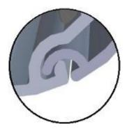
**Flush** the connector with either the top or bottom of the post.
