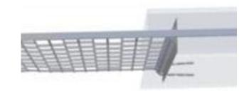
**Place** the V-stop flush with the front connector face of the trailing post.
